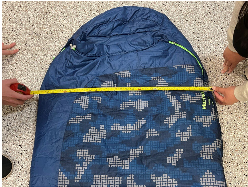
Figure 3: Measuring Width of Mummy Sleeping Bag at Single Widest Point
